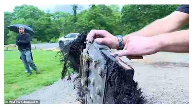
Above, more detail from the futuristic SpaceX trunk panel, fuzzed with burnt and frayed carbon fibers, bolted between heavy metal plates
